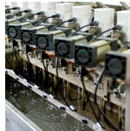
Hydrostatic pressure test-1
